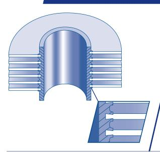
The fin strip is wound into a machined groove and securely locked into place by back filling with base tube material. This ensures that maximum heat transfer is maintained at high tube metal temperatures.
