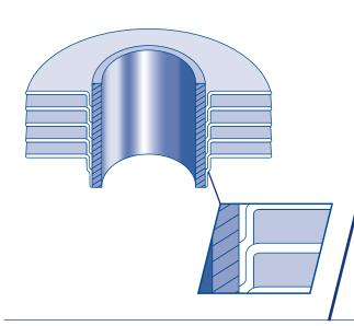
Manufactured in the same way as the 'L' fin type except that the fin foot is overlapped to completely enclose the base tube thereby giving excellent corrosion resistance. This type of tube is often used as an alternative to the more expensive extruded type fin in corrosive environments.
