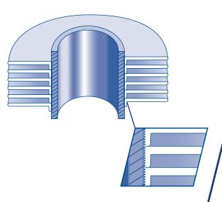
Manufactured exactly as the 'L' fin except that the base tube is knurled before application of the fin foot. After application, the fin foot is knurled into the corresponding knurling on the base tube thereby enhancing the bond between the fin and tube, resulting in improved heat transfer characteristics.
