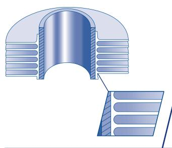
This fin type is formed from a bi-metallic tube consisting of an aluminium outer tube and an inner tube of almost any material. The fin is formed by rolling material from the outside of the exterior tube to give an integral fin with excellent heat transfer properties and longevity. Extruded fin offers excellent corrosion protection of the base tube.
