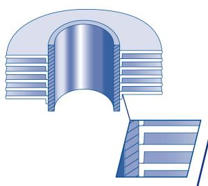
The strip material is subjected to controlled deformation under tension giving the optimum contact pressure of the foot of the fin onto the base tube thus maximising the heat transfer properties. The foot of the fin considerably enhances the corrosion protection of the base tube.
